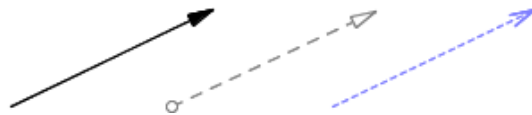
Figure B.6.: BPMN Connection types. From left to right: Sequence Flow , Message Flow , Association
